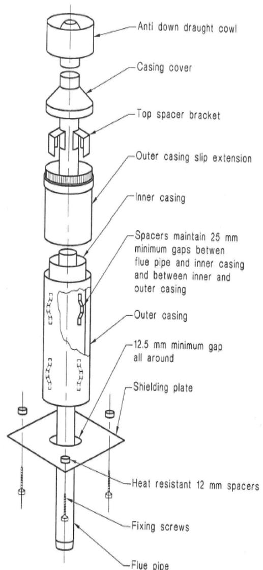
**WARNING:** The Fire and Flue System shall be installed in accordance with AS/NZS 2918:2001 Appendix F and the appropriate requirements of the relevant building code or codes. Firenzo/SFP Flue Kits or Davin Flue Kits must be used.
